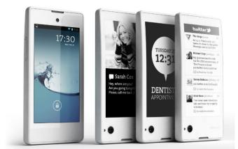
The device remains fairly unchanged from when we first saw it back at CES 2013. It still features a 4.3-inch 1280x720 LCD display on the front and a same-size 640x360 EPD on the back, providing what Yota calls an "always-on, low-power display."
