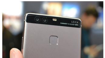
Reportedly the result of 3 years of co-engineering between the two companies, the dual cameras inside the P9 feature specially designed f/2.2 lenses, a pair of 12MP 1.25um Sony IMX286 sensors and a dual-LED flash. One camera captures RGB information while the other is monochrome, and the result is supposed to provide clearer photographs with brighter backgrounds, better contrast and better performance in low light environments.
