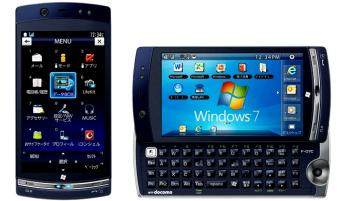
It's basically a PC inside a compact (measuring 125mm x 61mm x 19.8mm) design, with a 1.2GHz Intel Atom Z600 processor, 1GB of LPDDRR400 memory and 32GB of eMMC storage.
