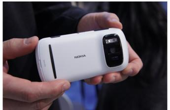
PureView technology uses "oversampling"-- taking image data from 7 neighbouring pixels and combining it into one pixel to generate a single 2/3, 5 or 8MP image (technically not 41MP, but still impressive for a mobile device).
