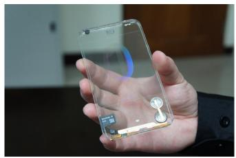
As seen on the website Mobile Geeks, the invisible smartphone is made from two sheets of Polyvision Smart Glass, an opaque privacy glass that turns transparent with the application of an electrical current.
