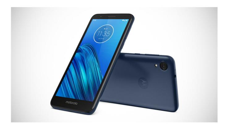
The E6 is smaller than last year's 5.7-inch E5, if with the same 1440 x 720 resolution, making the IPS LCD panel appear slightly sharper. The battery also sees a downgrade, being 3000mAh instead of 4000mAh, but it is actually removable. The processor is improved, being a Snapdragon 435 chip promising a 50% improvement over the Snapdragon 427 inside the E5, while RAM and storage remain identical at 2 and 16GB respectively.
