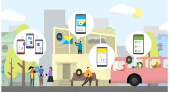
Named after the Eddystone Lighthouse in the UK, the beacon system uses Bluetooth to beam relevant data to mobile devices in range. It broadcasts either app data or web links, and makes use of one of two APIs to either find and ping nearby beacons (such as at a retail outlet) or send information when one is at a specific location (through latitude/longitude).
