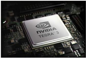
Nvidia claims the Tegra 3 provides up to x3 the graphic performance and 61% less power consumption over the Tegra 2, via 4-core 1.3GHz ARM Cortex A9 CPU, 12-core GPU and a 5th low-power "companion core" running low-intensity processes such as audio streaming, some video playback and standby modes.
