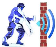
In concept Wi-Vi is similar to radar and sonar imaging, only using low-power wifi signals to track movement in closed rooms or behind a wall. The system requires 2 transmit antennas and 1 receiver, with one transmitter sending out a signal that is the inverse of the signal from the other.
