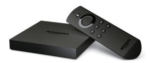
The Fire TV devices in question are upgrades of the <u>original STB</u> and the <u>Stick HDMI dongle</u>. The new Fire TV feature 4K/UHD resolution and HEVC (High Efficiency Video Coding) support, as well as more processing power, 802.11ac MIMO wifi and 8GB built-in storage (expandable to 128GB via microSD card slot).
