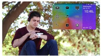
Designed to make (supposedly) better use of wrist real estate, the Rufus Cuff features a 3.2-inch display, TI Cortex A9 processor, 16/32/64GB storage, GPS, wifi and a 1175mAh battery. It runs on Android Kit Kat and offers fitness tracking features similar to other such devices through accelerometer, gyroscope and compass, as well as any number of smartphone apps and features.
