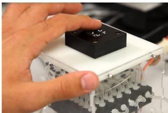
Braille displays and keyboards already exist but, being based on motorised pin systems, such systems tend to be heavy and expensive. The University of Michigan solution uses liquid or air to fill bubbles forming Braille symbols, making it both smaller (around tablet-size) and capable of showing more complex information than traditional devices.
