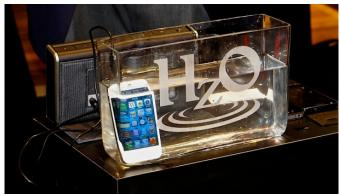
The technology consists of a nano-scale waterproof coat companies can apply to device components at manufacturing stage. It appears to work, too. At CES 2012, the company showed off the technology by dropping a working WaterBlock-treated iPod in a fishtank. The media player continued playing, even under water.
