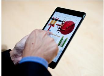
No longer the iPad3 but the "new" iPad features no enhancement more prominent than its Retina display with improved resolution ( $2048 \times 1536$  and 264 pixels per inch vs  $1024 \times 768$  resolution and 132 pixels per inch).
