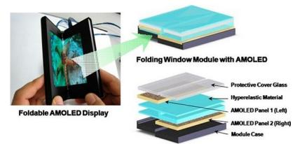
The prototype in question consists of x2 AMOLED panels with silicone rubber (a hyperelastic material), a protective glass cover and a module case. The display's folding radios is of just 1mm-- meaning the panels nearly touch each other when folded at a 180° angle.
