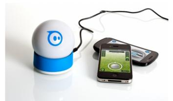
The Sphero looks unassuming-- it is basically a palm-sized white plastic ball. Inside, however, are a "smart robot" (with a gyroscope, compass and accelerometer), a multi-coloured LED (producing "thousands of colours") and a Bluetooth radio. Powering it is a rechargeable battery carrying up to 1 hour of juice.
