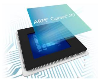
Designed for use in high-end embedded applications such as next-generation vehicles, connected devices and smart buildings, the M7 runs at 400MHz (in comparison the previous M4 runs at 168MHz), allowing for faster audio and image processing, as well as demanding embedded applications.
