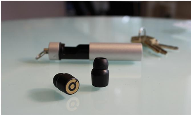
The tiny buds weigh all of 5g and measure 14mm wide and 20mm long. They connect to smartphones and other audio devices via Bluetooth (3.0/4.0) and carry 50mAh batteries promising up to 3 hours of playtime.
