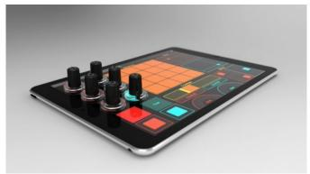
A creation of Dutch design company Tweetonig, the Tuna Knobs act as a radial stylus when attached on touchscreens via suction cap. The underside and soft-touch rubber grips on the knobs are conductive, meaning they only control virtual dials and knobs when touched by the users.
