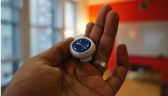
Meanwhile the Up Move is a small device similar to the Misfit Flash. Built out of anodised aluminium, it is designed to be kept in one's pocket, clasped to clothing (clip included) or slotted in a wrist strap accessory, and can track steps taken, activity and sleep.
