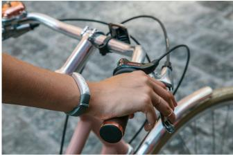
A successor to the Up24, the Up3 is the most sensor-heavy Jawbone fitness wearable yet. It features an tri-axis accelerometer, bioimpedance sensors (use tiny electric currents to measure heart rate, respiration rate and galvanic skin response), skin sensors and an ambient temperature sensor, and the company claims it automatically detects a wide range of activities, such as running, cross-training and sports.
