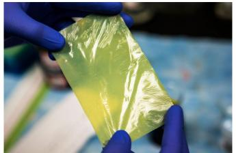
The solution is inspired by the battery fires that grounded Boeing 787 Dreamliners back in 2013. Lithium-ion batteries produce power by shuttling lithium ions from one electrode to the other, with a membrane blocking the shortest path between the two electrodes. However the lithium atoms might start creating fern-like structures (or dendrites) poking through the microscopic pores in the membrane, thus shorting out the battery.
