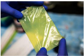
The solution is inspired by the battery fires that grounded Boeing 787 Dreamliners back in 2013. Lithium-ion batteries produce power by shuttling lithium ions from one electrode to the other, with a membrane blocking the shortest path between the two electrodes. However the lithium atoms might start creating fern-like structures (or dendrites) poking through the microscopic pores in the membrane, thus shorting out the battery.
