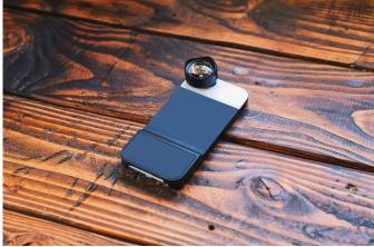
Described by the company as "the fastest way to take better pictures with your phone," the Moment Case features a rubberised grip on the back and securely holds Moment's own 18mm wide-angle and 60mm telephoto iPhone lenses via bayonet mount. However the most interesting addition is a hardware shutter button. Separately powered by a coin cell battery, it pairs with the iPhone via Bluetooth LE and provides DSLR-style fine-tuned shutter controls with half and full presses.
