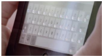
Described as a "morphing tactile surface," the technology uses "tiles" (Tactile Pixels) to turn specific areas of the screen into squishy tactile buttons via micro-fluid. Once the keyboard is not needed the keys disappear with the flick of a trigger. The technology is technically not too new, having made its first appearance back at CES 2013.
