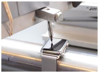
Apple uses two kinds of glass in the Watch-- the Sport features "Ion-X" glass (a material similar to Corning's Gorilla Glass), while the more expensive aluminium-bodied Watch and gold-plated Edition feature sapphire crystal. Consumer Reported tested both displays using the Mohs Hardness Scale, a 10-point mineral toughness test created by German geologist Friedrich Mohs back in 1812.
