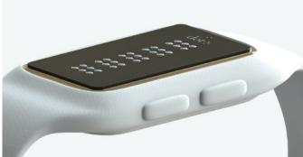
Instead of a display the Dot features a series of pins spelling 4 Braille characters at a time by rising and falling at custom speeds. The devices connects to smartphones via Bluetooth and provides regular smartwatch features (such as watch, alarm, messenger and navigation) as well as act as a Braille eReaders.
