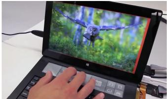
As Microsoft puts it, tablets have admittedly limited screen sizes, and as such the addition of a display to the keyboard extends available display real estate. Thus the DisplayCover has a 1280x305 resolution touchscreen extending the screen area of a tablet with a 10.6-inch display by up to 8%.
