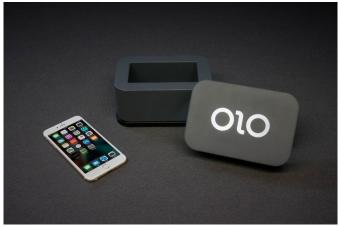
Described as a miniature stereolithography 3D printing system, the OLO is compatible with any smartphone with a display up to 5.8-inch in size, and essentially uses a combination of companion app (iOS and Android) and smartphone display to replace the projector component in a DLP printer.
