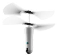
The ROAM-e features a twin rotor on the top and collapsible blades, making it easy to pack and carry in a bag. According to the company the drone features facial recognition able to detect users from up to 25m, ensuring they are always in shot.
