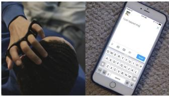
The Tap is made out of a soft foam material and slips on the fingers like a knuckleduster. It uses any flat surface-- "a table, a chair or even your body"-- and a unique input system able to turn 31 different taps into letters or numbers. Connectivity comes through Bluetooth and the makers say it is compatible with smartphones, tablets, wearable devices and even VR headsets.
