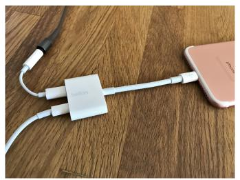
The Belkin 3.5mm Audio + Charge RockStar is a fairly self-explanatory accessory-- it is means to add a headphone jack to Lightning-only devices, while providing a source of data or power.
