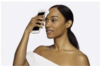
The SkinScanner uses a 30x magnification lens illuminated by 12 LED lights, as well as a moisture sensor. It is attaches to the iPhone camera, and is designed to be pressed directly up to the user's face. Pairing with the Skin360 companion app allows it to compare pore size, moisture, wrinkles and other such factors to other users on the system in the same age range, before giving the user a score out of 100.
