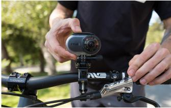
Launched back in November 2017 for iDevices, the Rylo sits somewhere between the low-cost Insta360 One and high-end GoPro Fusion cameras. It features a pair of 208-degree lenses and auto-stabilisation technology, and records video as a 4K resolution 360-degree sphere. Video transfers between camera and app take place not via wifi but through a traditional transfer cable.
