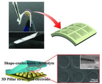
The bendable batteries use "fluid-like polymer electrolytes" instead of traditional liquid electrolytes poured into cases. According to the Korean Science Ministry fluid-like electrolytes are not only flexible but also more stable, reducing explosion risks.
