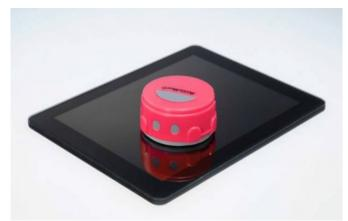
Looking like a palm-sized Roomba robot, the AutoMee S trundles on 5 tires (3 for maneuvers, 2 for cleaning) over devices, with sensors making sure the little robot does not fall off the edges while performing its duties.
