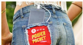
A University of Southampton development, the Power Pocket consists of multiple "thermocouples" making a thermomaterial small enough to stitch into clothing. Taking advantage of the difference between body and outside temperatures (the so-called Seebeck effect), the material generates voltage and current when heat flows through the warm (body-facing) and cool (outside-facing) sides of the material.
