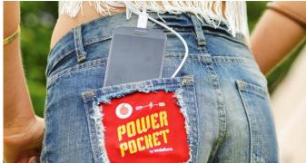
A University of Southampton development, the Power Pocket consists of multiple "thermocouples" making a thermomaterial small enough to stitch into clothing. Taking advantage of the difference between body and outside temperatures (the so-called Seebeck effect), the material generates voltage and current when heat flows through the warm (body-facing) and cool (outside-facing) sides of the material.
