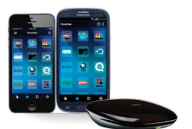
The Ultimate Hub is originally part of the <u>Harmony Ultimate and Smart Control product</u> <u>packages</u> first seen on April 2013. A puck-sized device similar to the Harmony Link, the Hub receives RF and wifi signals before it issues commands to up to x8 devices via IR and Bluetooth.
